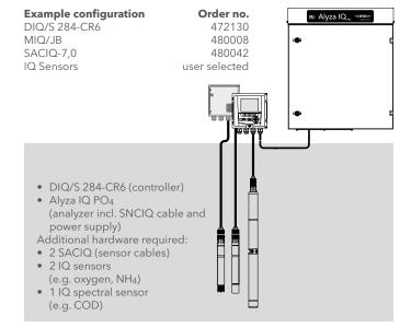
Neither example 1 nor example 2 needs a power supply module MIQ/PS, as the Alyza IQ provides 10W to the systems.
